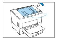
3 Press the top cover release button and open the cover.
